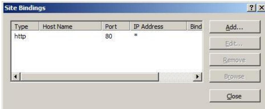
The default settings for a new binding are set to HTTP on port 80. Select **https** in the **Type** drop-down list. Select the self-signed certificate you created in the previous section from the **SSL Certificate** drop-down list and then click **OK**.
