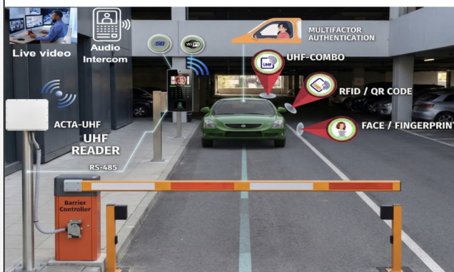
Car Parking Solution Connection Diagram
